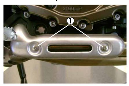
Using a PH3 phillips driver, remove these (2) OEM fasteners.
