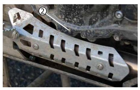
2 Put the AltRider guard in place and using a PH3 phillips driver, tighten the OEM fasteners down.
